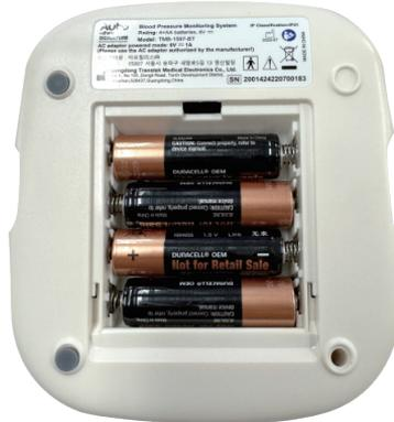
Check if the batteries are properly inserted into the back of the blood pressure monitor.
